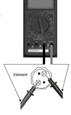
Disconnect wires from the element terminals. See OHMS Resistance Table – Page 45
